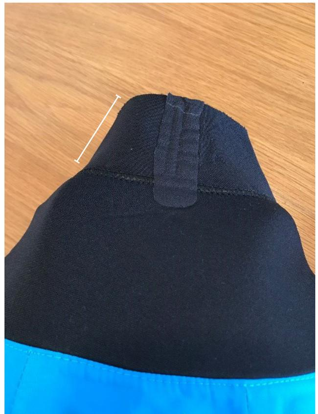
You can simply cut around the upper band of the neoprene seal with a sharp pair of scissors, approximately 3-5mm at a time, until you can get the seal over your head and it still fits snugly on your neck. The neoprene won't split, so long as the edge is cut smoothly, and the seam won't run as it is taped.
