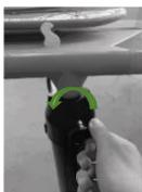
When you first start inflating it's best to have the lever at the back of the pump turned to the right. In this setting the pump will work on double action, pumping on both the up and the down stroke. When this gets too difficult twist the lever to the left and the pump will swap to single action. In this setting the pump will only act on the down stroke which will make it much easier for you and your arms.
