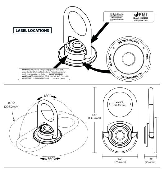
Tensile Strength (UTS): 10,000-lbf (44kN)
