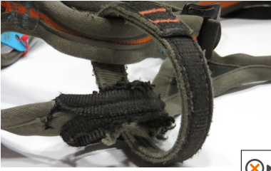
• Worn tie-in point
