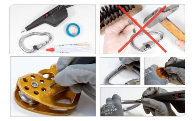
You can use adhesive tape on the areas where the rope does not run.
