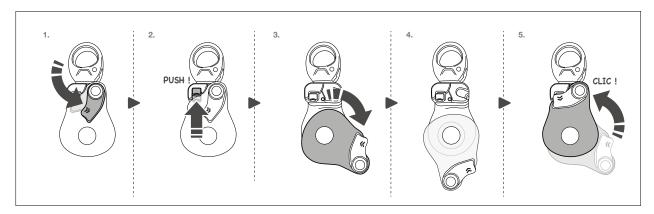
• Check the condition and function of the locking system (marks, deformation, dirt, effectiveness of the return spring(s)).
