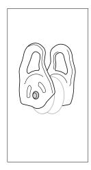
• Check the condition of the rivets (marks, deformation, cracks, corrosion, absence of play...).
