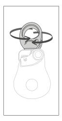
• Check the condition (marks, deformation, cracks, wear, corrosion) and the rotation of the swivel in both directions.
