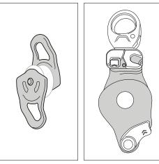
$\bullet$  Check the condition of the side plates (marks, deformation, cracks, wear, corrosion).
