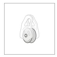
• Check the condition of the sheave (marks, deformation, cracks, wear, corrosion, absence of foreign bodies...).
