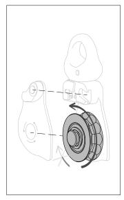
• Check the condition of the ratcheting wheel (marks, deformation, cracks, wear, corrosion...). Verify that the sheave turns in the desired direction and blocks in the other direction.
