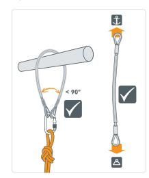
Performance and ultimate strength will be reduced by larks footing / choking around anchor points, storage and ageing due to use, etc. (list not exhaustive).
