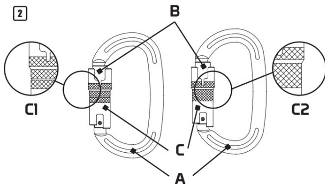
EN: (A) Body, (B) Gate, (C) Automatic gate locking device: (C1) TWIST-LOCK, (C2) AUTOBLOCK.
