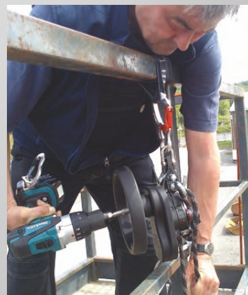
Lifting the casualty with battery screw driver
