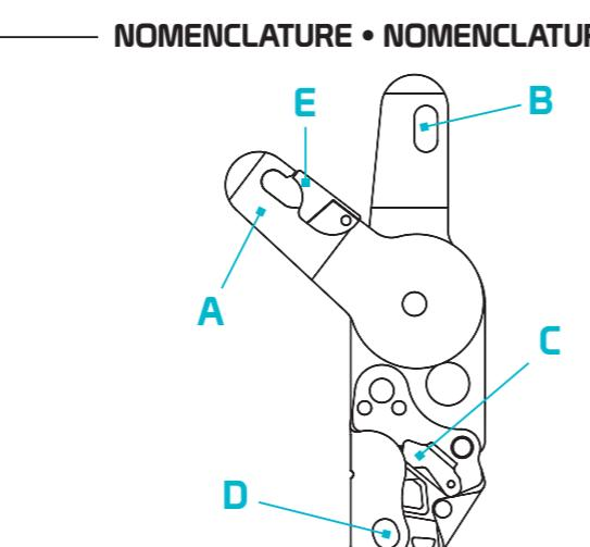
**EN:** (A) Sheave plate, (B) Main eyelet, (C) Rope clamp, (D) Secondary connection holes, (E) Safety gate.
