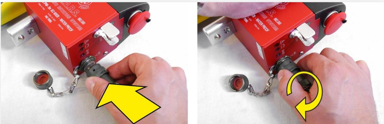
FIG.22 Connection of the battery charger connector
