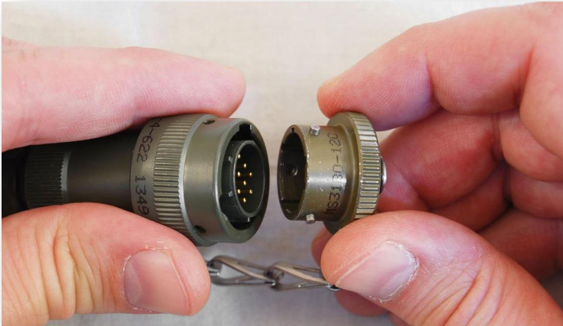
FIG.21 Battery charger connector
