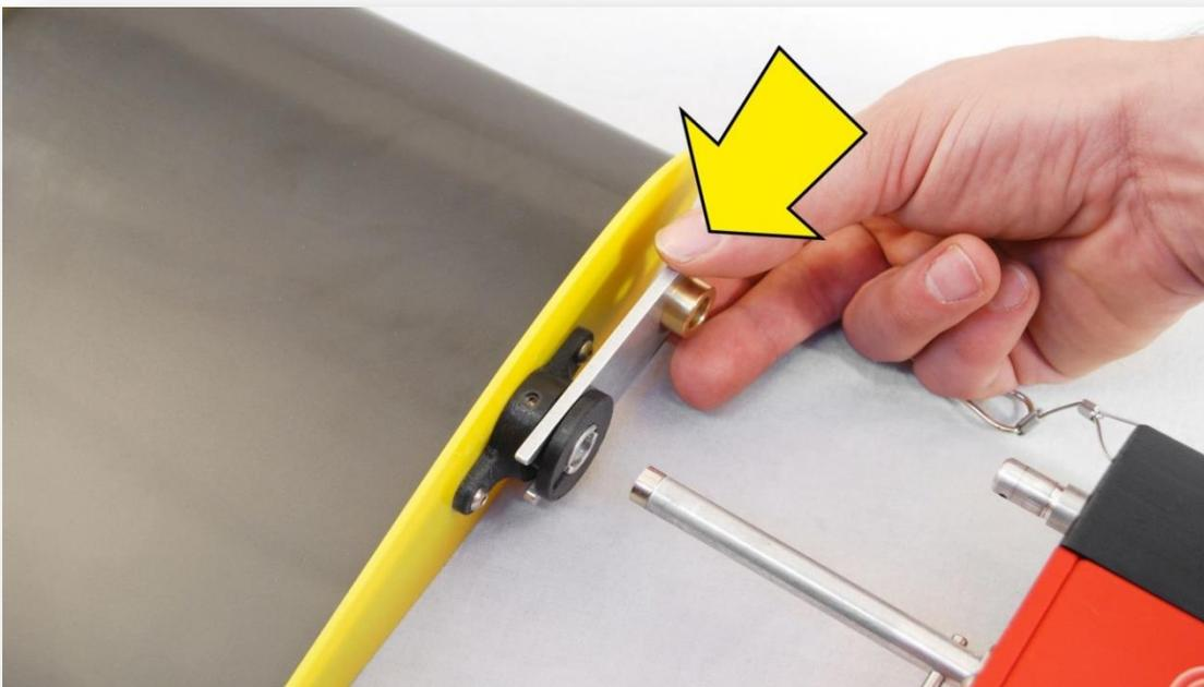
FIG.26 Fitting the fork
