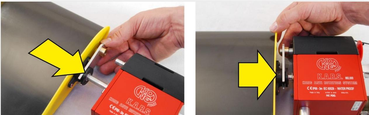
FIG.28 Inserting the wing in the KARS body
