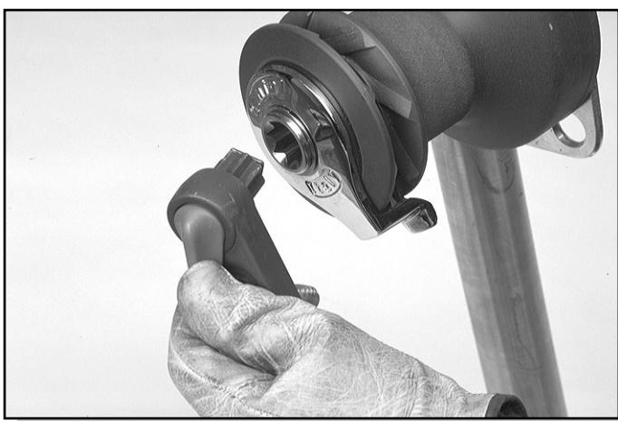
After checking the correct placement and the stability of the rescue stand insert the hand levers in the winch by rotating the little lever at the top of the handle to mate the safety board (fig. 12). To take them off work backwards.
