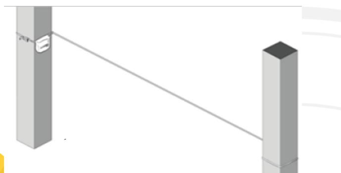
3. Clamped to structure at both terminals
