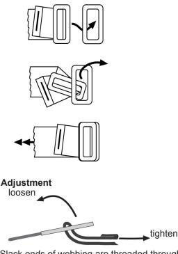
Slack ends of webbing are threaded through plastic loops to keep them out of the way.
