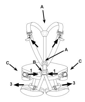
Step into harness, fasten and adjust in the order 1 - 2 - 3 in the diagram. If necessary the rear D-ring may be adjusted up and down by use of the rear buckle
