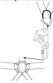
Attach the small triangular screwlink just below the D-ring to the top hole of the chest ascender. Make sure all screwlink connectors are correctly fastened with no thread visible.
