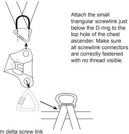
Use an 8mm delta screw link connector to attach the lower hole of the chest ascender in to the webbing loop behind the central D-ring.
