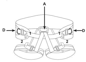
Step into harness, fasten and adjust in the order shown in the diagram.
