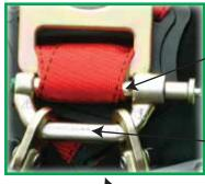
Locking pin inserted through harness webbing under dorsal D-ring
