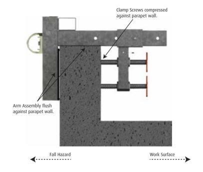
If Parapet Anchors are to be used in Fall Prevention applications, continue with the following guardrail installation instructions:
