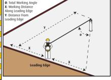
For example, if the anchorage connector is 6' from the leading edge (Y), the working distance (X) is 8' in each direction from the perpendicular, which translates to a 53° working angle.
