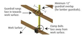
6. Install all guardrails. Guardrails may be compatible snap-on metal rails, or 2" x 4" or 2" x 6" construction grade lumber. If using lumber guardrails, guardrails MUST overlap a minimum of 12" at each end between consecutive guardrail posts.
