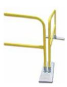
4. For all baseplates, tighten set-screws/reinstall locking pins. Ensure guardrails are firmly installed and do not move. Ensure all toeboards will run parallel with guardrails. Insert all  $2^{"}x4^{"}$  toeboards into attachment points.
