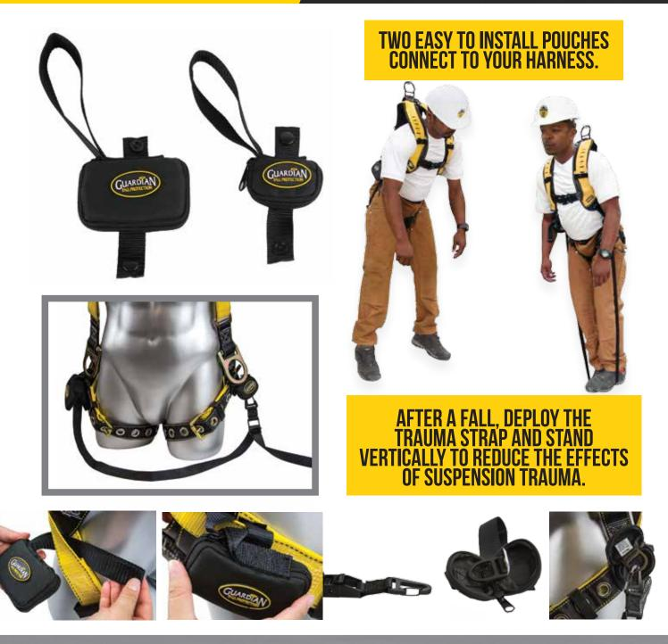
AN IMPORTANT PART OF ANY RESCUE PLAN. EM 381-1-1 STATES "ALL FULL BODY HARNESSES SHALL BE EQUIPPED WITH SUSPENSION TRAUMA PREVENTERS SUCH AS STIRRUPS, RELIEF STEPS, OR SIMILAR IN ORDER TO PROVIDE SHORT TERM RELIEF FROM THE EFFECTS OF ORTHOSTATIC INTOLERANCE. MATERIAL: NYLON, POLYESTER, AND STEEL CAPACITY: 420 LBS.
