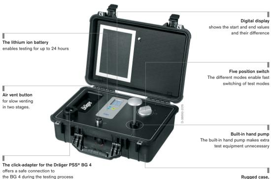
Rugged case, IP54 certified against dust and water (with locked lid), ideal for use on-the-go
