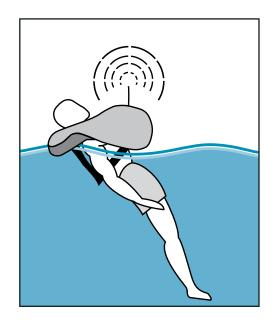
The lifejacket's sculpted bladder combined with the placement of the sMRT positions the PLB's antenna for optimum performance.
