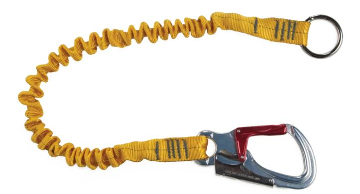
This strong tether, made from 1-inch tubular web with a built-in bungee, works as a "live bait" water rescue attachment to your PFD. As a connection between a PFD and a line, the tether enhances attachment options in rescue situations. Comes with brite double-locking connector. Rated strength: 11 kN (2,473 lbf)
