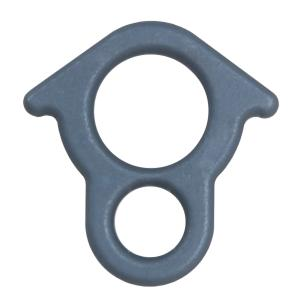
Machined from 9.5-mm (3/8-in) aluminum, this compact figure 8 descender works well with escape lines or other small diameter ropes where minimum size and weight are the primary requirements. The rounded edges reduce sharp bends. The large carabiner hole accepts a wide variety of carabiners and helps prevent binding. The Survivor 8 features a hard anodized finish in a dark gray for users who require a non-reflective surface.
