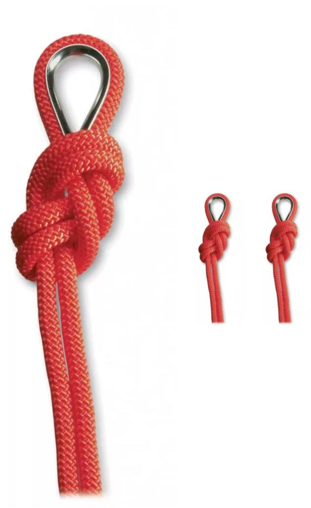
Rope thimbles protect rope from wear whenever you have a fixed loop in the end of the rope-whether the rope is tied, spliced, or swaged. These thimbles are stainless steel for high strength and resistance to corrosion. Unlike plastic thimbles, they are less likely to break leaving sharp edges exposed.
