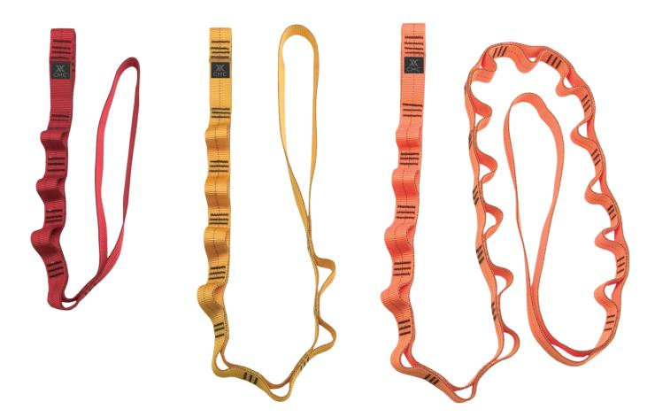
Made of 1-inch (25-mm) mil-spec tubular web, these straps allow you to tie into your anchor with just the right length of web. They're also handy for clipping several carabiners into one anchor point. Pocket stitching breaks at 5 kN (1,100 lbf). Available in 3 sizes.
