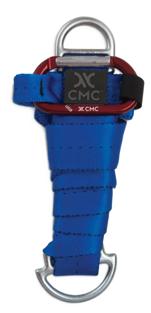
Our Load Release Strap makes sizing and tying a load-releasing hitch dependable, fast and easy. Constructed from the same high-strength web and hardware as our Anchor Straps, the larger D-ring on the load end has enough space for multiple carabiners. The wide web and multiple wraps provide a high degree of control during release. The strap comes assembled with our red ProTech™ Oval Carabiner.
