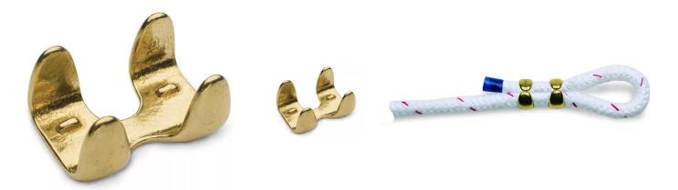
Quick and easy to install, requiring only a mallet to fold the prongs over on the doubled rope. This clamp slips at 800 lbf and fits 1/2-inch and 3/8-inch Ladder Line.
