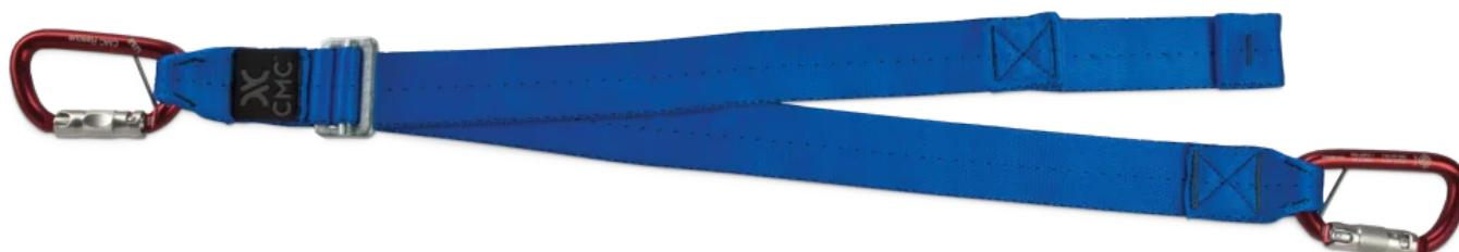
This is the only Pick-Off Strap with two carabiners incorporated directly into the strap, which reduces the overall weight. We use the same high-strength, mil-spec web and adjuster hardware as our original Pick-Off Strap. The web begins to slip through the buckle at 17-18 kN (3,800-4,000 lbf). The two ProTech<sup>TM</sup> Auto-Lock Carabiners with keeper pins are UL Classified to NFPA 1983 – Technical Use.
