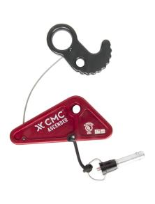
The CMC Ascender rope grab utilizes a spring-loaded cam to facilitate progression on life safety rope. Widely used by rescue teams as a rope clamp for an attachment to a litter harness tender line, as a travel restrict rope grab, ascending rope, and other applications where a mechanical rope grab provides greater efficiency.
