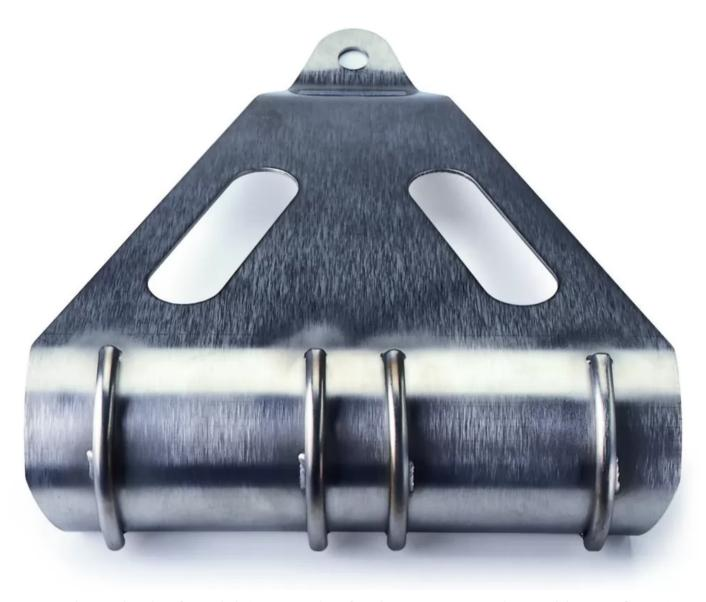
The Entry-Ease changes the edge of a manhole into a smooth surface that a person or stretcher can slide over. It fits entries as small as 18 inches (46 cm) in diameter and also works on railings, pipes, ladder rungs, or other surfaces with high friction or that may damage a lifeline. The stainless steel Entry-Ease may be your only option in a location with low overhead clearance.
