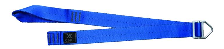
We developed the Adjustable Litter Strap because it allows minor adjustments to be made while the litter is being carried. Quickly releasing the buckle extends the strap, preventing the rescuer from being pulled down with the litter. Sewn loop strength exceeds 36 kN (8,093 lbf). The strap can also be used for pick-offs.
