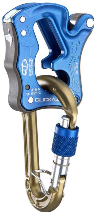
CLICK UP is a belay device with manual braking, especially designed for crag climbing. It can be used with  $\varnothing 8.6 \div 10.5$  mm single ropes. It is compact and lightweight and allows for belaying a leader and belaying a top-rope climber with both hands handling the rope, or for lowering the climber.
