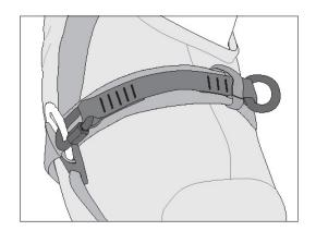
ACCESS RING Ref.2046 Aluminum alloy connection ring. Diameter: Int.34 mm - Ext.54 mm
