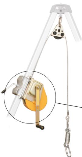
Rescue device **ref.0284 or 028401** may be easily installed (Cable length: 20 m or 25 m). Working load limit: 140 kg. Supplied separately together with pulley and connectors.
