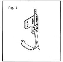
Attach sleeve to leg iron with sleeve loop facing outside of pad (away from the wearer's leg) using the fasteners enclosed. Insert barrel nuts from inside of leg iron. See Fig. 2a & 2b ('right' climber shown). Note: Two fasteners (screws, star washers & barrel nuts) must be used to secure each sleeve to each leg iron. Do not over tighten, torque to 25 inch pounds maximum.
