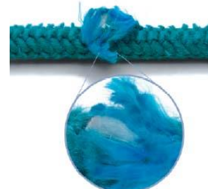
Rope with Broken or Cut Strands
