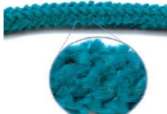
Rope with Excessive Abrasion Wear
