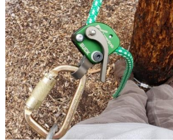
LeverGrab positioned on left side with Carabiner reversed (Left hand adjustment set-up)
