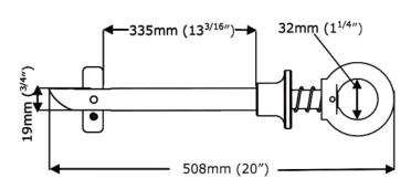
Girder & Concrete Anchors are a quick and easy portable anchorage solution and can be used in the vertical and horizontal plane. These anchors are operated by using two fingers to pull back the red collar. This action retracts the retention bar, allowing the device to be inserted into the anchor hole. Once the device is in position, the red collar can be release, causing the retention bar to engage, fixing the device in position.
