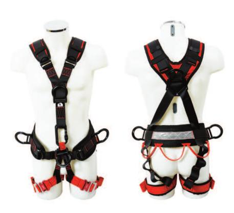
Rear dorsal attachment point for fall arrest and rescue of user. Front 'D' for fall arrest and rescue of user. The soft loops that link the belt to the chest can be used to facilitate abseiling, ascending and descending and the attachment of another person for rescue. Side 'D's are for work positioning and the comfort belt with tool loops for lumber support.
